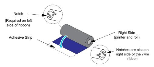
Verify that the ribbon and empty ribbon core have notches on the left side of the ribbon cores as shown above. If they do not, see Loading Non-Zebra 300 Meter Transfer Ribbon.
