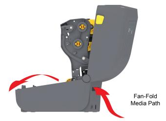
2. Adjust the media guide stop position with the Slide Lock (gray). Use a piece of the fan-fold media to help set the stop position. Push gray locking slide on the left-hand roll holder towards the back of the printer to lock the roll holder position. Pull it forward to release the lock.
