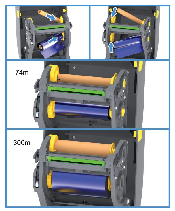
**3.** Attach the ribbon to the take up core. Use the adhesive strip on new rolls; otherwise, use a thin strip of tape. Align the ribbon so that it will be taken straight onto the core.
