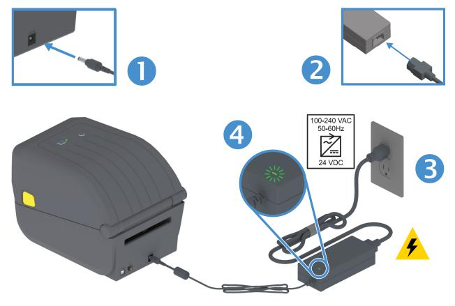
**Important** • Ensure the appropriate power cord with a three (3) prong plug and an IEC 60320-C13 connector are used at all times. These power cords must bear the relevant certification mark of the country in which the product is being used.
