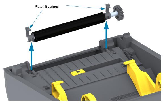
**4.** Slide the gear and the two (2) bearings off the shaft of the platen roller.
