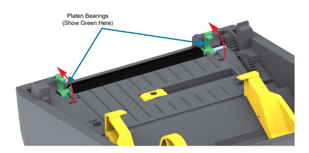
**3.** Lift the platen out of the printer's bottom frame.
