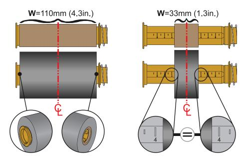
3. Place the adapter with an empty core on the take-up spindles and the adapter with the ribbon roll on the lower supply spindles. The right side of the core adapter fits on the cone tip on each of the spring loaded right side spindles. Continue pushing the adapter onto right side spindle and swing the adapter onto the left side spindle hubs. Rotate the adapters and hubs until the until notches on the adapters flange align and lock ton the left spindles hub spokes.
