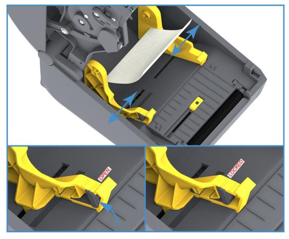
**3.** Insert the media through the slot at the rear of the printer and place the media between the media guide and roll holders.
