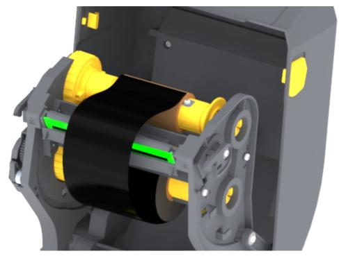
**6.** Turn the ribbon take-up hub with the top moving toward rear to remove slack from the ribbon. Rotating the hub helps to finish aligning the take up ribbon position with the supply ribbon roll. The ribbon should be wound, at minimum, one and a half times around the take-up ribbon core.
