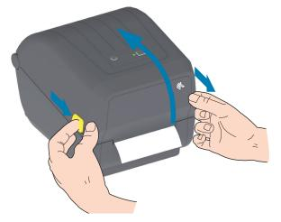
2. Open the media roll holders. Orient the media roll so that its printing surface will face up as it passes over the platen (drive) roller. Pull the media guides open with your free hand and place the media roll on the roll holders and release the guides. Verify the roll turns freely. The roll must not sit in the bottom of the media compartment.
