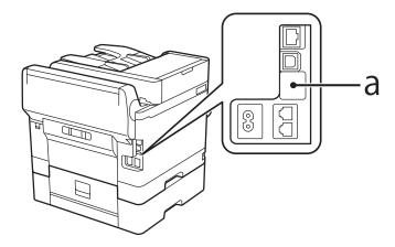
Connect the USB cable for the authentication device to the service port.
