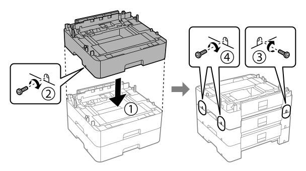
11. Lower the printer gently onto the optional paper cassette units aligning the corners, and then secure them with the screws using a screwdriver.
