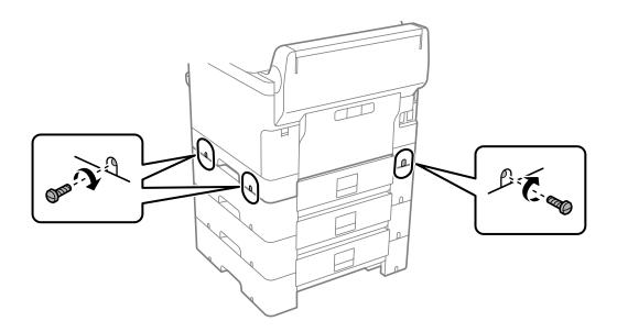
13. Attach the part that you removed in step 4 to the back of the lowest optional paper cassette unit.
