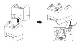
Connect one end of the included DC cord to the DC connector OUT of the first battery charger and connect the other end of the DC cord to the DC connector IN of the second battery charger.
