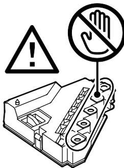
5. Place the removed waste cartridge on a level surface.
