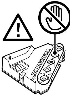
6. Place the removed waste cartridge on a level surface.
