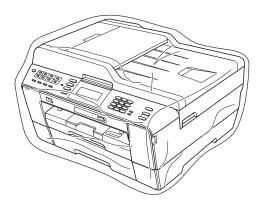
10 Pack the machine and the printed materials in the original carton with the original packing material as shown below. Do not pack the used ink cartridges in the carton.
