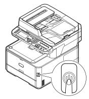
**3** Plug one end of the Ethernet cable into the network interface connection on the back of the machine.
