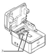
**12** Press the top cover open button (8) and open the top cover.
