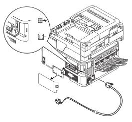
**4** Plug the other end of the Ethernet cable into the hub.
