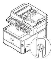
**3** Plug one end of the USB cable into the USB interface connector on the back of the machine.
