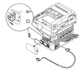
**4** Plug the other end of the Ethernet cable into the hub.
