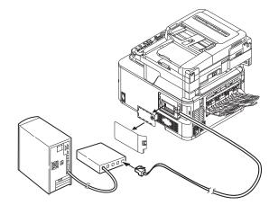
**5** Hold down the power switch for approximately one second to turn on the power.
