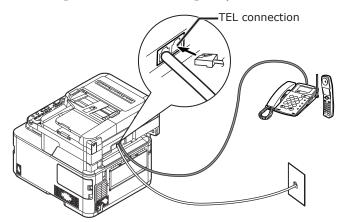
The telephone that is connected to the machine is called an external telephone.
