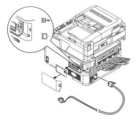
**4** Plug the other end of the Ethernet cable into the hub.
