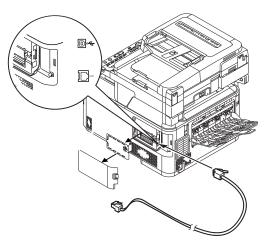
Plug the other end of the Ethernet cable 4 into the hub.
