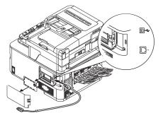
**4** Plug the other end of the USB cable into the computer's USB interface connector.
