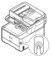
**3** Plug one end of the USB cable into the USB interface connector on the back of the machine.
