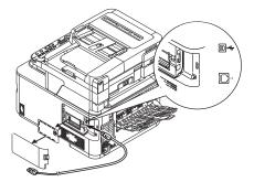
**4** Plug the other end of the USB cable into the computer's USB interface connector.
