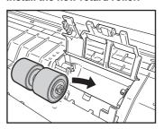
Slide the securing lever for the retard roller to the right, and lower it backward.
