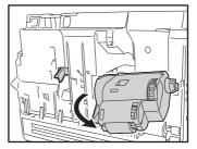
5 Attach the right joint of the new feed roller.
