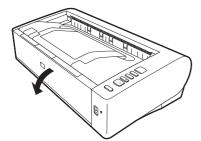
3 Switch the eject method based on the type of document you are scanning.
