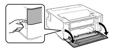
2. Lower the output switch lever.
