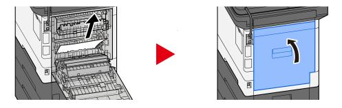
Open the Rear Cover 2 and remove the jammed paper.
