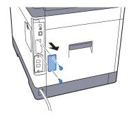
4 Insert the SD/SDHC memory card into the SD/SDHC memory card slot.
