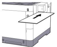
When the paper is inserted all the way in, stapling takes place.
