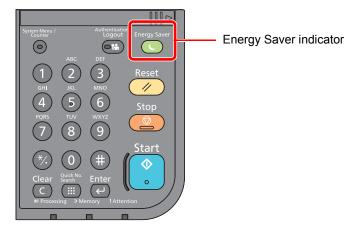
If print data is received during Sleep, the machine automatically wakes up and starts printing.
