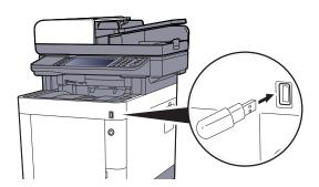
2 When the machine reads the USB memory, "Removable Memory is recognized. Displaying files. Are you sure?" may appear. Select [**Yes**] to display the removable memory screen.
