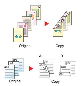
Produces two-sided copies from one-sided originals. In case of an odd number of originals, the back side of the last copy will be blank.
