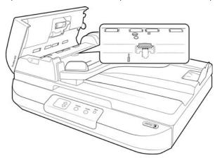
2. Squeeze the plastic clamp that holds the pad assembly in place.
