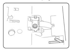
6. Place the new ADF pad in the scanner on top of the tension spring.
