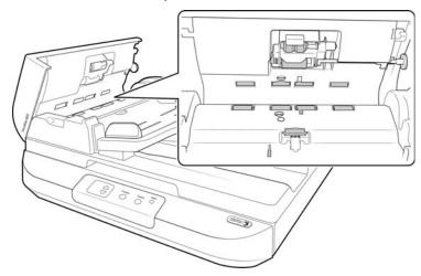
3. Wipe the feed roller from side to side. Rotate the roller to clean its entire surface. The feed roller is located in the underside of the ADF door.
