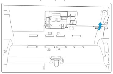
4. Remove the roller from the scanner and discard it, it cannot be repaired.
