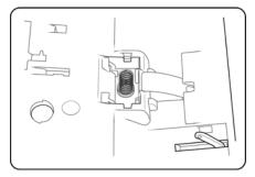
5. Place the new tension spring in the scanner.
