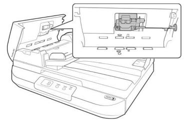
3. The roller is held in place with a lock tab that rotates to lock and unlock it. To unlock the tab, rotate it upward until the small lock flange is completely free.
