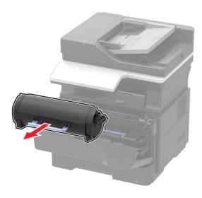
**3** Remove the used imaging unit.
