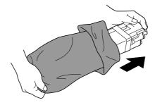
10. Hold the photoconductor unit with both hands, and then shake it twice as shown in the illustration.
