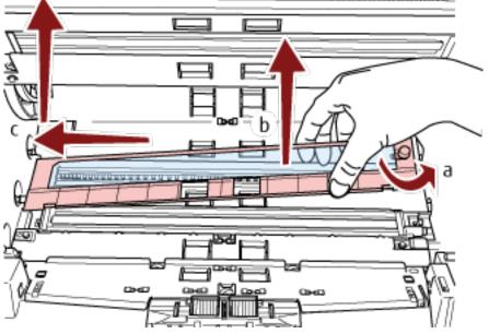
**a** Loosen the screw until the glass can be lifted.
