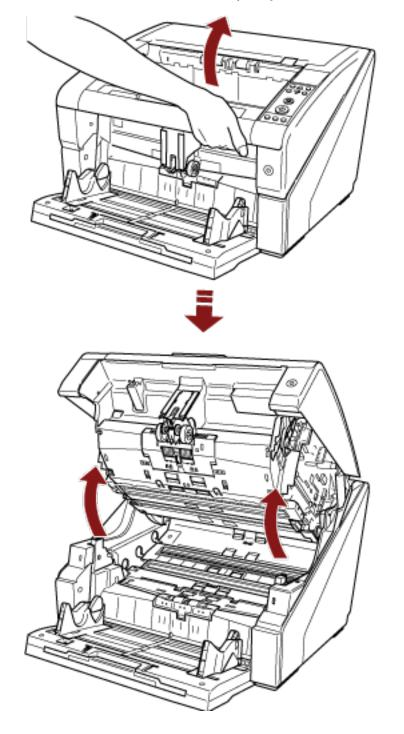
2 Grab the ADF release tab and lift it up to open the ADF.
