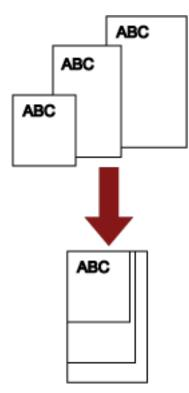
2 Place the documents on the hopper and adjust the hopper side guides to the widest document in the batch.
