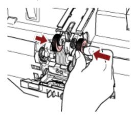
a Place the pick rollers (× 2) on the shaft.
