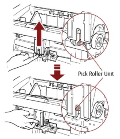
The pick roller unit will click into place. The hopper moves up to the feeding position.
