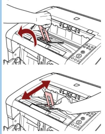
To scan documents longer than A3 size, pull out the hopper extension and stacker extension all the way. Also, make sure not to pull up the paper stop.
