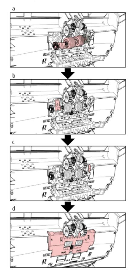
5 Install a new separator roller on the scanner.
