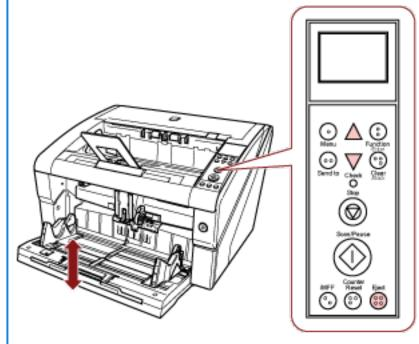
When [Hopper Level] is displayed by shortcut key, the screen returns to [Ready] after a certain period of time. This period of time can be configured in [18: Operation Panel Timeout] of the operator panel.
