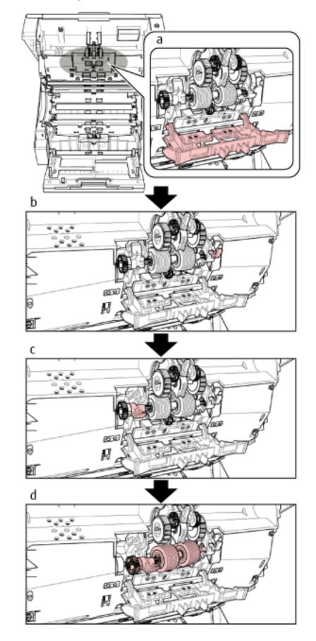
4 Remove the separator roller from the scanner.
