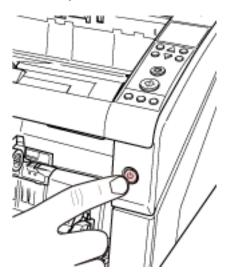
The power is turned on, and the power button lights in blue. Note that the following screen is displayed on the operator panel LCD during initialization.
