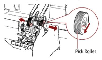
5 Install a new set of pick rollers (× 2) in the scanner.
