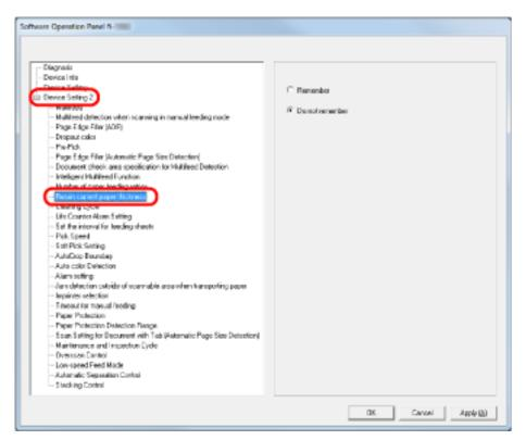
**3** Specify whether or not to memorize the paper separation force setting of the operator panel upon turning the power off.
