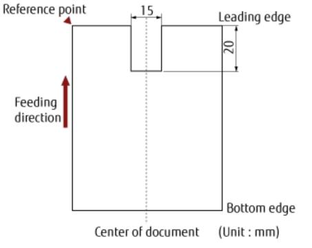
The following is a typical form of a Job Separation Sheet.
