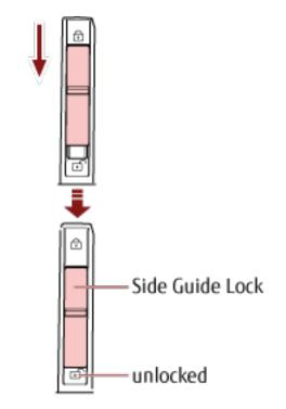
**2** Move both hopper side guides towards the center while pressing the side guide clutches.
