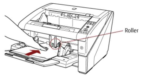
The document is picked, scanned, then ejected onto the stacker.
