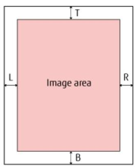
T: Top = 0 to 15 mm B: Bottom = -7 to 7 mm R: Right = 0 to 15 mm L: Left = 0 to 15 mm (in 1 mm increments) The specified area is filled in the same color as the background.
