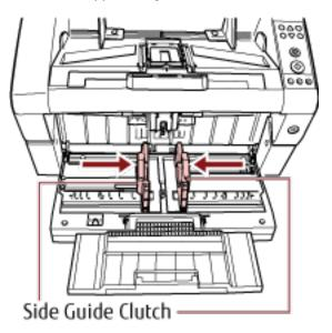
3 Release the side guide clutches.Both hopper side guides will now move in conjunction with each other.
