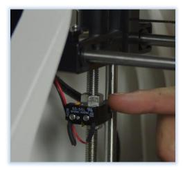
• The x axis sits on top of these Z limit switches until the nozzle reaches the home position (or the auto leveling code is executed); at this point the nozzle touches the bed and releases the limit switches, signaling that the extruder has reached "home"
