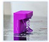
• Support material can be broken away after the print job is finished.
