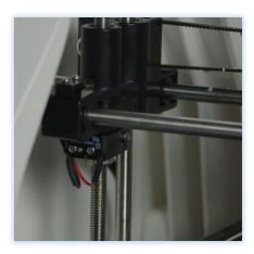
• It is very important to make sure that the coupler nuts that these limit switches sit on are always seated in the cavity of the X brackets on both sides (They may come off durring transportation or rough handling) otherwise the auto leveling feature will not work.
