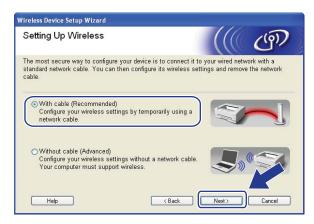
8 Read the **Important Notice**. Check the box after you confirm the wired setting is enabled, and then click **Next**.
