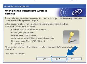
If you want to configure your machine for the wireless network you have been using, write down your wireless network settings before configuration.
