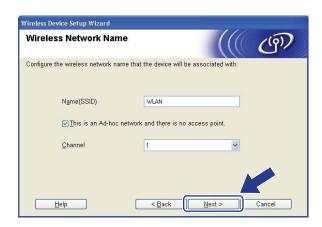
If your network is not configured for Authentication and Encryption, the following screen will appear. To continue configuration, click **OK** and go to step **6**.
