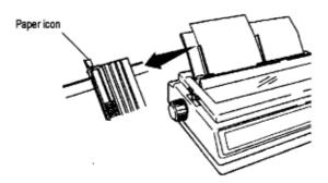
4. Insert a piece of single-sheet paper and adjust right paper guide to width of paper.
