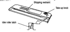
5. Place ribbon cartridge in printer: pins on either end of car-tridge fit in notches in plates on either side of printer platen. Push down on cartridge until it clicks into place (see diagram on cartridge).
