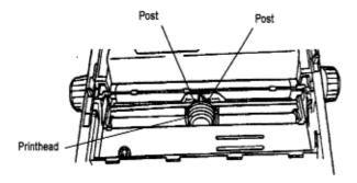
3. If you are replacing the ribbon: slide ribbon off printhead posts, remove cartridge from printer, and discard used cartridge.
