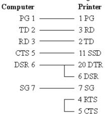
IBM 9-Pin Serial Cable Configuration
