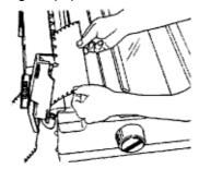
9. Close rear cover, turn printer on and press FORM FEED button to load in paper.
