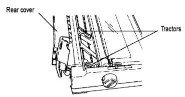
3. Open both tractor covers and pull forward on right-hand lock lever to unlock right tractor.
