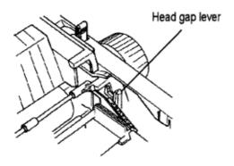
To adjust the head gap, open the access cover. The blue head gap lever is located on the right side of the printer. Use the recommended head gap from the table below to ensure the best print quality and proper paper feeding.
