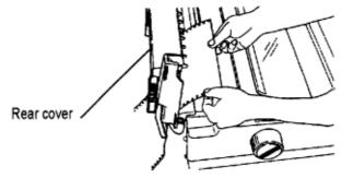
5. Slide right-hand tractor to adjust it to width of paper, then set paper on tractor pins at either end and
