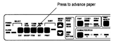
9. Set Top of Form (TOF) by holding PARK button while pressing appropriate MICRO FEED button. Paper will advance up or down in direction of arrow on button youre pressing. (For more details, see Setting Top of Form later in this chapter.)
