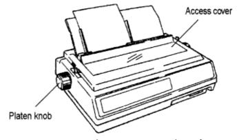
3. If necessary, open access cover and remove any torn pieces from around carriage.
